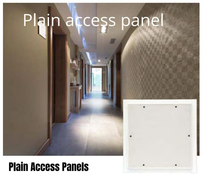
**Characteristics:** Non-fire rated Plain aluminum access panel frames are electrostatic powder coated white, with Regular Grade Gypsum board facing, Providing easy access to gypsum ceilings. Each panel features a push-catch closing mechanism, with door retaining safety cable and hook. Applications Suitable for applications where access to services above gypsum ceiling are specified.
