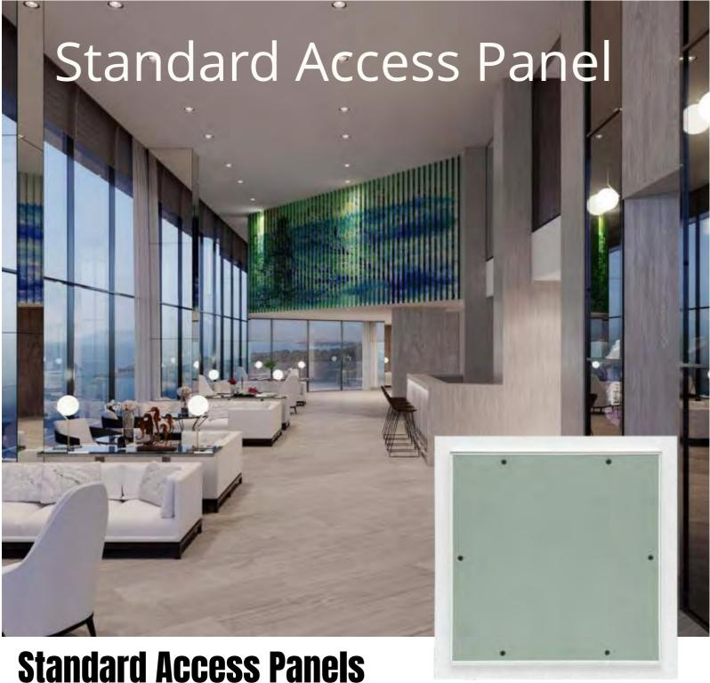
Characteristics: Non-fire rated standard aluminum access panel frames are electrostatic powder coated white, with MR Grade Gypsum board facing, Providing easy access to gypsum ceilings. Each panel features a push-catch closing mechanism, with door retaining safety cable and hook. Applications Suitable for applications where access to services above gypsum ceiling are specified.
